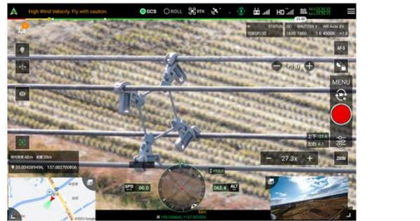
Tokyo-based Sensyn Robotics has announced enhancements to its inspection system, POWER GRID Check. A business application developed to aid in monitoring and maintaining overhead power transmission facilities, POWER GRID Check enables automatically navigated drones to inspect steel towers and transmission lines.
